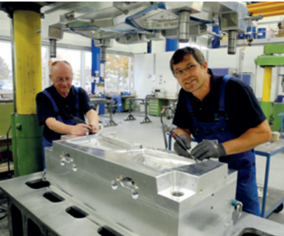
Peter Trexler (left) and Hans Wurm spot-grinding a mould. Photo: BBG
